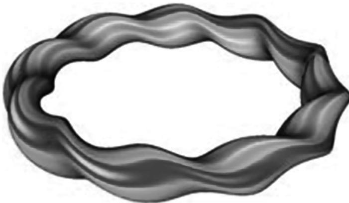
**FIGURE 23.1** Illustration of GTC 3D mode structure for the  $n = 1$  global Alfvén eigenmode in the large helical device (LHD) stellarator. (From D.A. Spong, *Phys. Plasmas* 22, 055602, 2015.)
