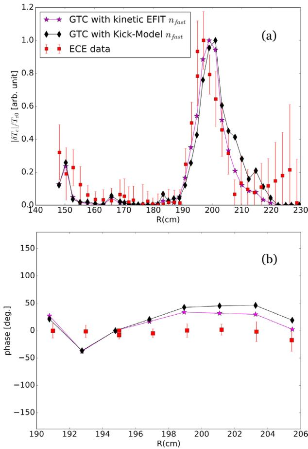
**Figure 11.** Comparison of GTC simulation data, after being processed through the synthetic-diagnostic-platform, to experimental ECE data for DIII-D #159243 at 805 ms. (a) Radial structure of  $|\delta T_e|/T_{e0}$ . (b) The phase profile relative to  $R = 195.0$  cm.
