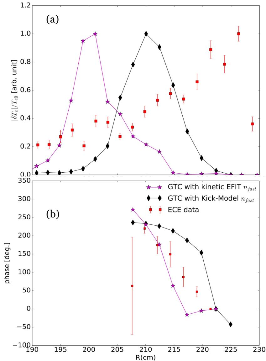
**Figure 13.** Comparison of GTC simulation data, after being processed through the synthetic-diagnostic-platform, to experimental ECE data for DIII-D #159243 at 805 ms. (a) Radial structure of  $|\delta T_e|/T_{e0}$ . (b) The phase profile relative to  $R = 221.4$  cm. The measured  $n = 6$  TAE ECE frequency is 98.9 kHz (plasma frame) and the GTC calculated value is 95.2 kHz.
