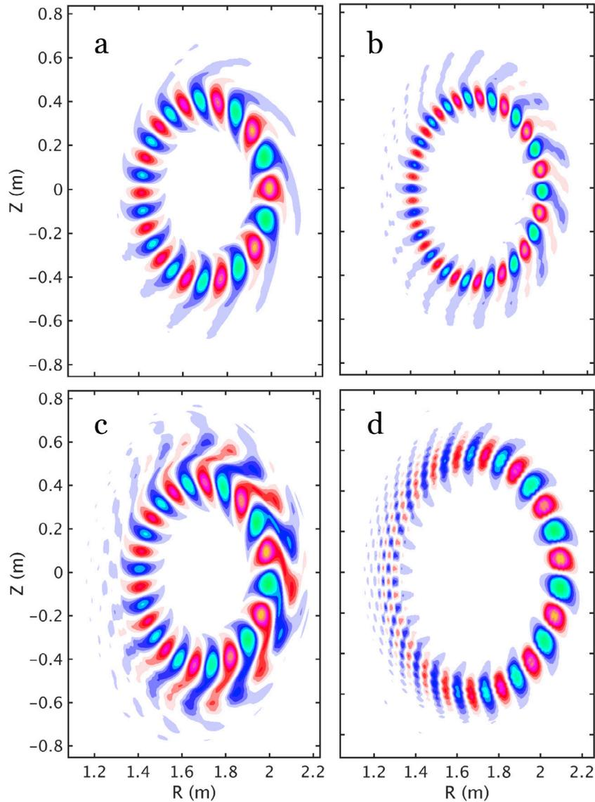
**Figure 7.** Perturbed electrostatic potential from GTC simulations of DIII-D shot 159243.00805. ((a)–(b))  $n = 4$  and  $n = 6$  simulations, respectively, using a fast ion density profile calculated from kinetic EFIT. ((c)–(d))  $n = 4$  and  $n = 6$  simulations, respectively, using a fast ion density profile calculated from the kick model.
