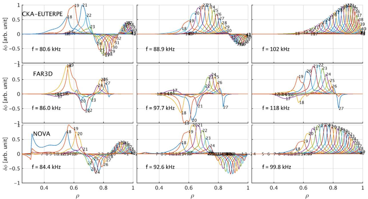
**Figure 10.** Radial TAE mode structures from TAE frequency scan using fast ion density calculated from the kick-model. (Top row) CKA-EUTERPE runs with  $f = [80.6, 88.7, 102]$  kHz. (middle row) FAR3D eigenvalue runs with  $f = [86.0, 97.7, 118]$  kHz. (bottom row) NOVA frequency scan with  $f = [84.4, 92.6, 99.8]$  kHz. In the figure, frequencies increase from left to right.
