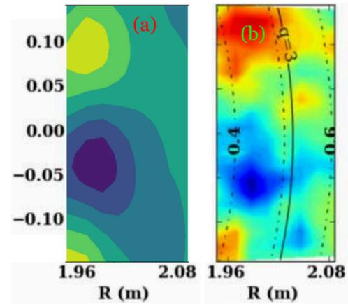
**Figure 12.** Comparison of  $n = 4$  RSAE mode GTC simulation data and experimental ECEI data for DIII-D #159243 at 807.3 ms. 2D structure on a poloidal plane of  $\delta T_e/T_{e0}$  for (a) GTC simulation data, after being processed through the synthetic-diagnostic-platform, and (b) experimental ECEI data.
