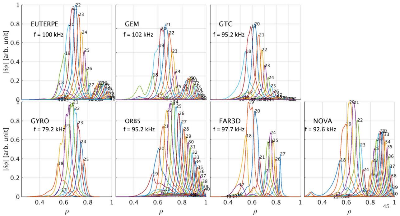
**Figure 9.** Radial structures of the poloidal harmonics of the electrostatic potential for the  $n = 6$  TAE, using the kick model fast ion density profile, for DIII-D shot 158243 at 805 ms. The simulated TAE frequency for each code is written in each panel.
