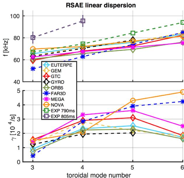
**Figure 4.** Linear dispersion relation calculation for RSAE in DIII-D shot 158243 at 805 ms. (a) Real frequencies. (b) Growth rates. The plot markers are diamond, star, and circle for the gyrokinetic, kinetic-MHD hybrid, and perturbative eigenvalue codes, respectively.
