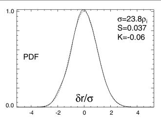
FIG. 2. Probability density function of test particle radial displacement (solid line) is very close to a Gaussian (dotted line).  $\sigma$ , *S*, *K* are, respectively, the standard deviation, skewness, and kurtosis of the measured data.
