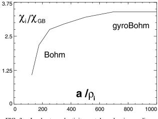
FIG. 3. Ion heat conductivity vs tokamak minor radius.
