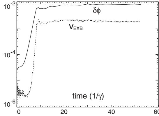
**Figure 2.** The volume-integrated fluctuation intensity ( $\delta\phi$ ) saturates in magnitude as the self-generated zonal flow ( $V_{E \times B}$ ) grows to a saturated amplitude. The radial spreading of turbulence occurs from approximately  $t = 8/\gamma$ , while the volume-integrated fluctuation intensity stays approximately a constant in time.
