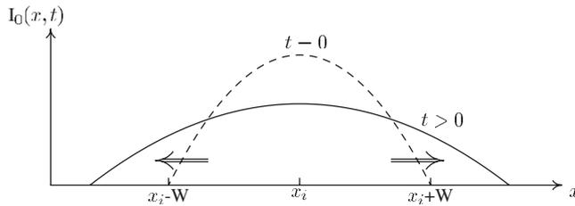
Figure 3. Equation (5) describes a propagating localized front-like solution.
