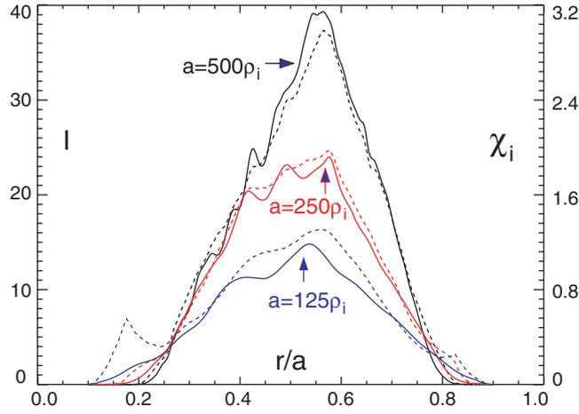
**Figure 5.** Fluctuation intensity profiles ( $I$  in —) and ion thermal diffusivity ( $\chi_i$  in ····), both in gyroBohm units after nonlinear saturation for  $a/\rho_i = 125, 250$  and  $500$ : as the system size gets larger, the extent of radial spreading of turbulence into the linearly stable zone gets narrower relative to the system size. It scales with the ion gyroradius  $\sim 25\rho_i$  [31].
